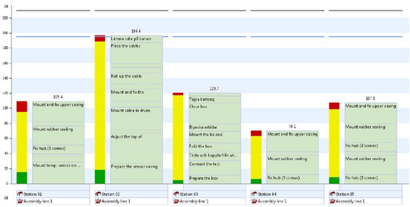
Image Caption: When rebalancing and optimizing a production line or work cell, value-added and non-value-added activity for each work station is instantly updated and displayed.
