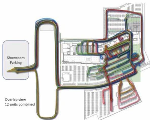
*Vehicles were moved more than two miles through multiple staging areas during the reconditioning process prior to creating a new streamlined process.*
