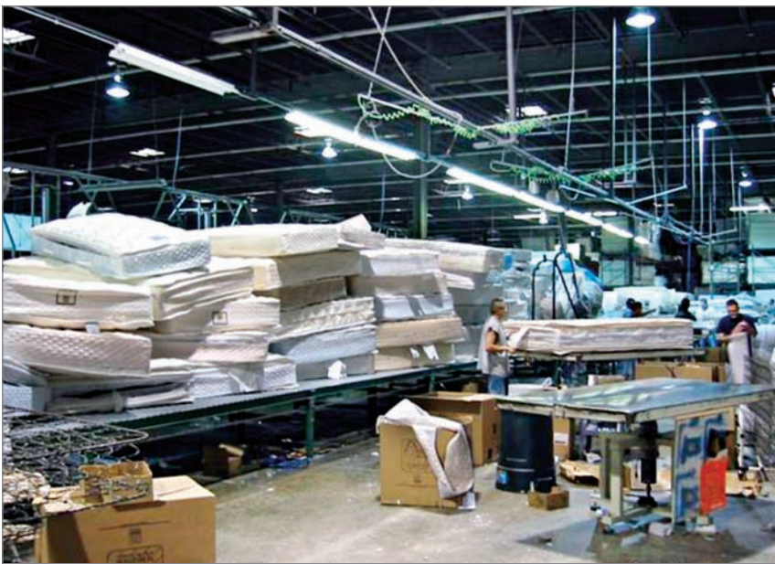
Stacks of work in process are clear evidence of overproduction — a type of waste that involves making products that no one has ordered
